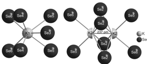
Figure 2 Selenide coordination spheres of both crystallographically different K^+ cations in the crystal structure of K_3Lu_7Se_{12} .
