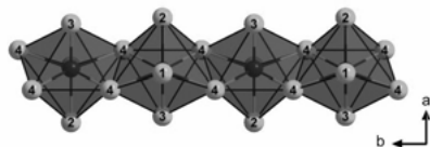
Figure 2 Strands of edge-connected [\text{TmF}_7]^{4-} polyhedra according to 1\text{D}-[\text{Tm}(\text{F}1,2,3)_3^{t/1}(\text{F}4)_{4/2}^e]^{2-} propagating along the b -axis in the crystal structure of \text{K}_2\text{TmF}_5 .
